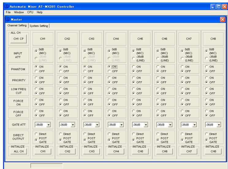
The AT-MX381 SmartMixer's channel settings appear in columns with the channel number at the top. The first column lists the items that can be configured for each channel. In the upper left corner is a button that allows channel one's settings to be copied to all of the other channels. Across the bottom of the window are "Initialize" buttons. When clicked, these will set the selected channel or ALL channels to their factory default configurations.
