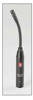
ES935SC6 is a wide-range miniature condenser microphone with a cardioid polar pattern and an integral mute switch/ LED. It is designed for quality sound reinforcement, professional recording, elevision and other demanding sound pickup applications. The small-diameter gooseneck design permits highly flexible positioning while maintaining a smooth, well-contoured appearance. An included snap-on foam windscreen effectively reduces wind noise and "popping."
