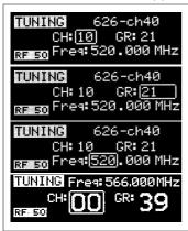
In this menu channel/group and frequencies can be setup. The name of the group is shown on the top right of the display. *SYNC* group is a quick self-settable channel synchronized by receiver (with SYNC group, on the top right of the display is shown the name of the synchronized receiver).
