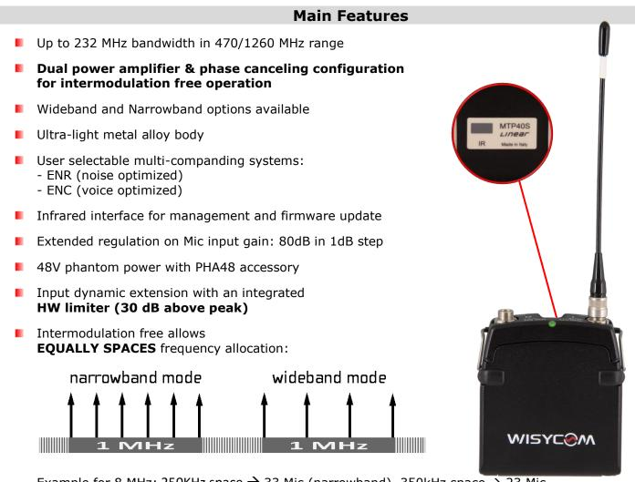
Example for 8 MHz: 250KHz space ightarrow 33 Mic (narrowband), 350kHz space ightarrow 23 Mic
